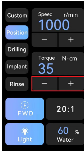
Fig. 10 Adjusting the upper limit of torque
