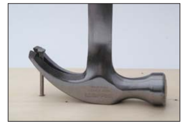
Figure 12. A claw hammer uses class I lever mechanics, with the handle one lever, the head of the hammer as the fulcrum, and the claw as the short lever applied to the nail. The Physics Forceps uses a similar action to remove a tooth.
