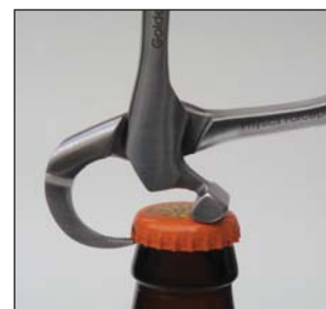
Figure 4. Physics Forceps applies the mechanical advantage of a first-class lever, similar to that of a bottle opener.
