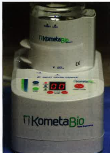
Figure 5. The Smart Dentin Grinder is a self-contained unit, consisting of a motor and a disposable chamber.
